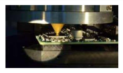
SQUID Sensor analysing the current track on assembled PCB (Magnetic microscopy)
